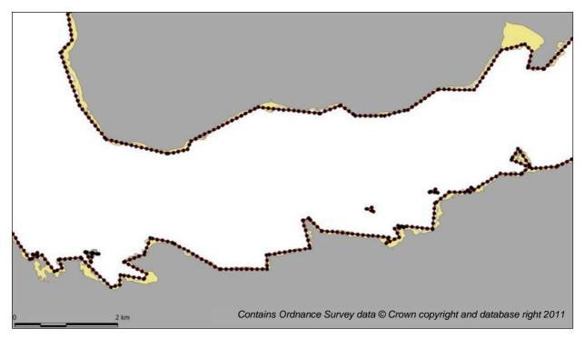
**Figure 4.** Virtual Observation Points (VOPs) every max 100m along a simplified low water coastline. Example shown is Loch Scridain, Mull.
