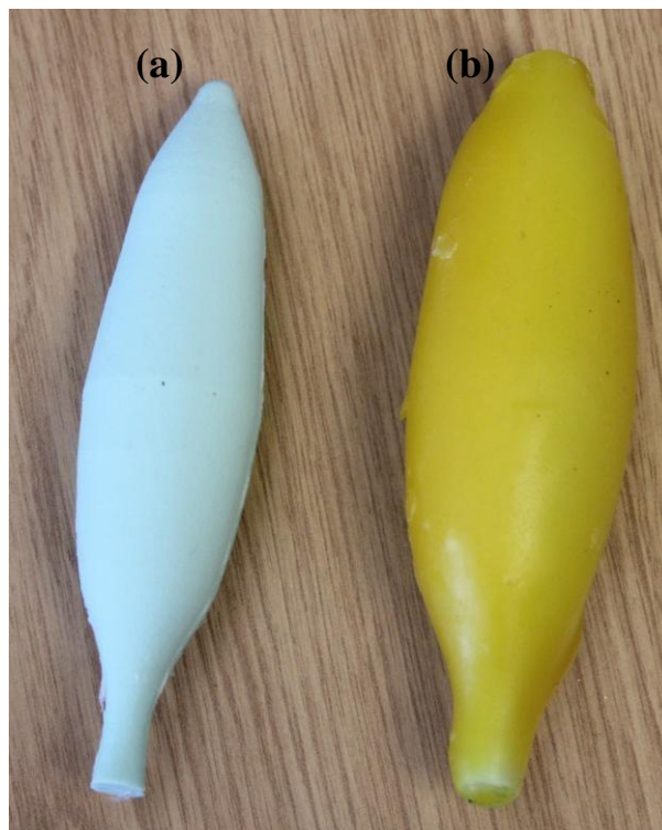
Figure 3. Scale replicates of (a) a juvenile grey seal body core and (b) a juvenile grey seal with a blubber layer. The body core measure 13 cm in length.
