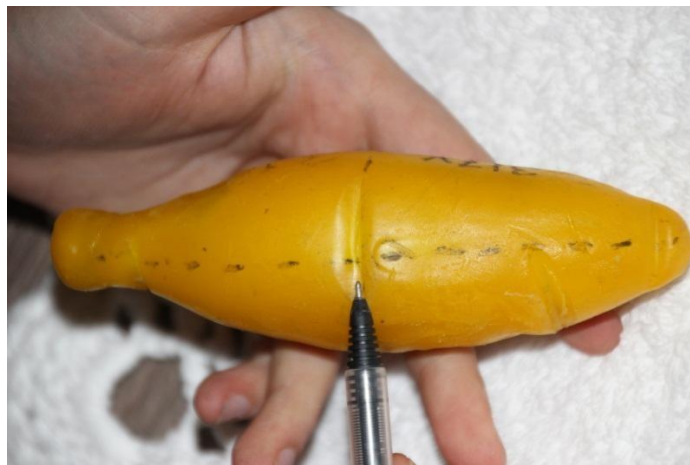
Figure 15. Figure shows the damage inflicted on the seal model by the collision with the Voith-Schneider Propeller
