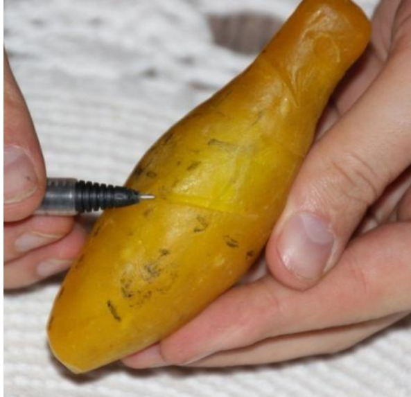
Figure 12. An example of damage resulting from a model passing through an open propeller. Note three separate impact marks: one indicated by the pointer, one on the front of the seal model and one at the rear. None of them resembled a spiral, curving wound and all were notably superficial with none cutting deeply into the wax layer.
