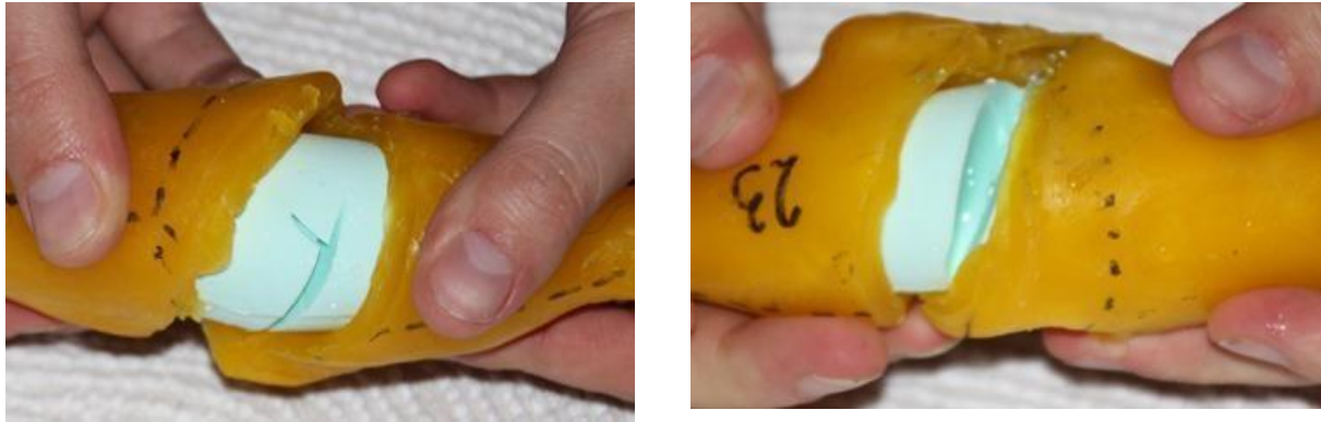
Figure 8. Examples of cuts to the silicone core of seal models resulting from blade impacts
