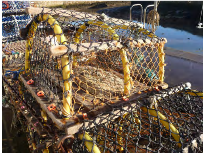
Fig 20: Parlour creel with rubber coating on steel frame
