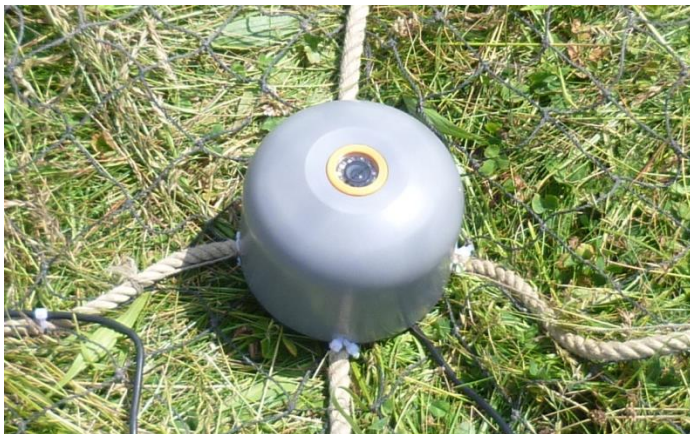
Figure 8. One of 8 underwater video cameras positioned within nets to monitor the frequency of seals and salmon entering modified and unmodified chambers of both control and modified nets
